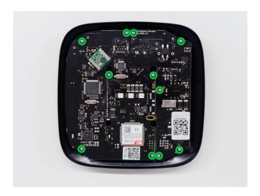
**6.** Carefully remove both boards, keeping them in the same plane and not disconnecting them. There is a connector between boards: do not break it.
