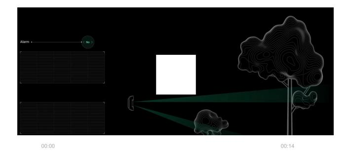
MotionCam Outdoor features two independent IR sensors, the signals of which are analyzed by a two-stage LISA algorithm. As soon as both IR sensors detect movement, LISA performs correlation and spectral analysis of the signals, which allows you to instantly distinguish between real threats and interference.
