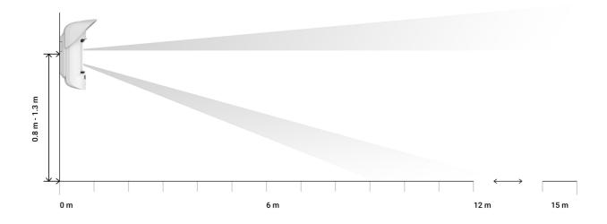
The detection distance is adjusted using the **Detection Distance** scrollbar on the rear panel of the detector. When choosing the installation location, consider the maximum detection range of the detector. It depends on the sensitivity, the position of the Detection Distance scrollbar, the type and speed of the person's movement (running, walking), and the ambient temperature.
