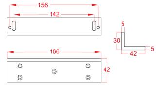
• Z-Brackets for armature plate
