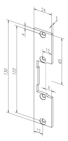
Short flat striking plate with latch bolt aperture.
