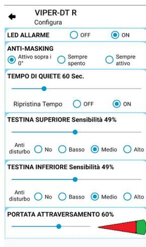
Figure 4 - Sensor setup
