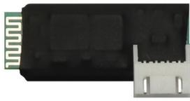
BT-LINK-S2 is an accessory for outdoor sensors series (VIPER, VIPER-DT, MOSKITO, KAPTURE), which allows the use of the VIEW SENSOR software on a mobile device in BT wireless connection with the DUEVI sensor.
