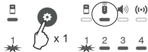
The numbers of the free positions (with no key fobs enrolled) are lighting in green, and those with already enrolled key fobs – in red. The currently selected position number is blinking.
