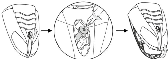
2. Remove the light pipe, undo the screws and remove one by one the metal and the plastic covers protecting the battery and the electronic parts.
