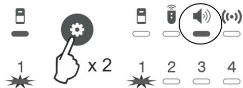
The BRAVO panel supports operation with one outdoor sounder, which can be enrolled to position 1.
