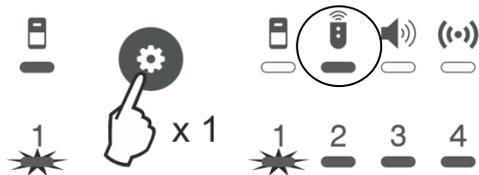
The numbers of the free positions (with no key fobs enrolled) are lighting in green, and those with already enrolled key fobs – in red. The currently selected position number is blinking.
