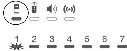
The numbers of the free zones (with no detectors enrolled) are lighting in green, and those with already enrolled devices – in red. The currently selected zone number is blinking.
