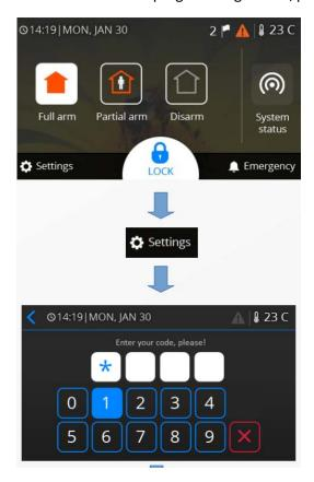
The keypad will simulate the engineer/manager menu just like in all other Eclipse keypads:
