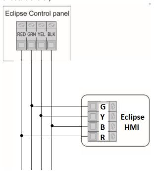
The initial version of the Eclipse HMI has the following labeling of the BUS terminals – PWR+/- (R and B respectively) and A/B (Yellow, Green). Please, follow the example picture below in order to attach the keypad to the Eclipse panel properly.
