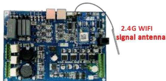
When using wireless routing module, please install 2.4G WIFI signal antenna correctly, and the antenna should not be in contact with the metal to ensure that the module signal can be received at a long distance.
