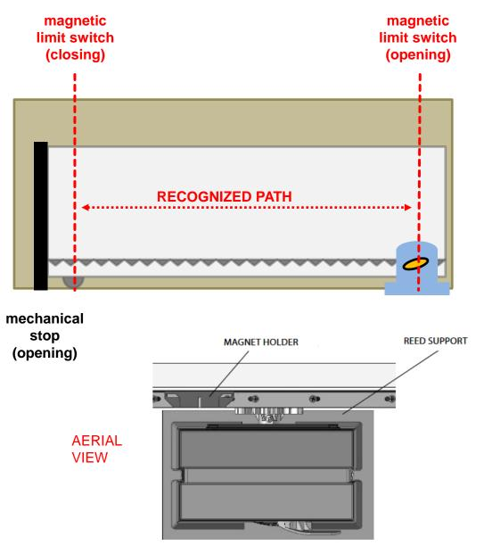
**NOTE:** The magnets position is adjustable, it can be moved forwards/backwards as well as laterally and its plastic or even on the metal bracket fixed to the gear rack. The same goes for the magnet sensors of the gate operator, opening and closing. The recommended distance is less than 2 cm.
