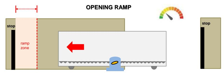
exact point for the gate leaf to start slowing down the speed
