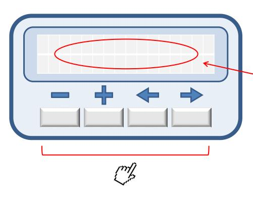
We use the <- (left) y -> (right) buttons to navigate in the function menu. While the + (plus) y - (minus) buttons are used to increase or decrease the value of each functionality.
