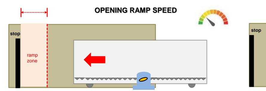
exact point for the gate leaf to start slowing down the speed
