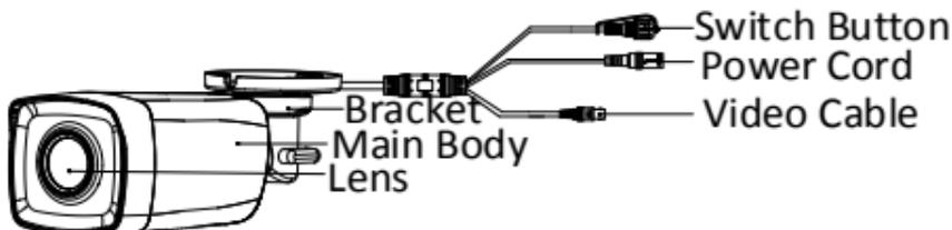
Figure 1-2 Overview of Camera Model with F
