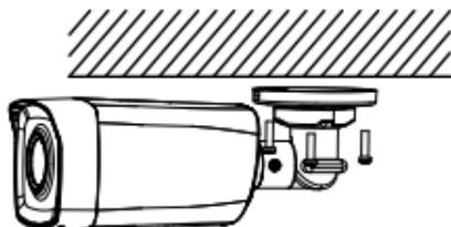
Figure 2-1 Secure the Camera on the Ceiling
