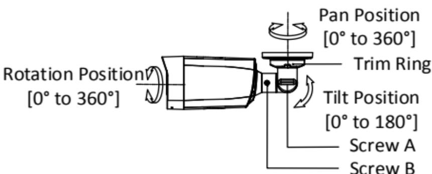
Figure 2-2 3-Axis Adjustment
