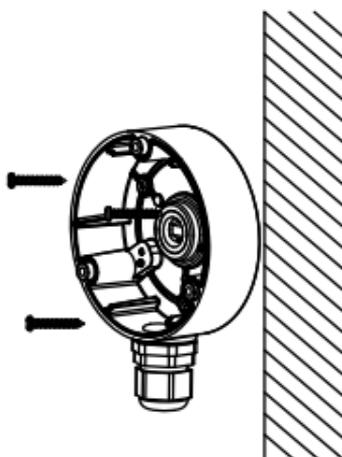
Figure 2-5 Secure the Junction Box on the Wall
