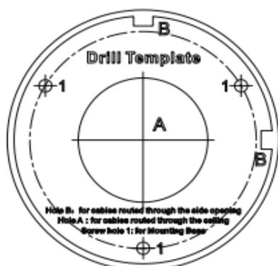
Figure 2-3 Drill Template for Junction Box
