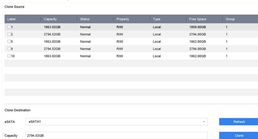
**Figure 16-9 HDD Clone**
