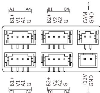
Figure 3-1 Terminals of Indoor Station
