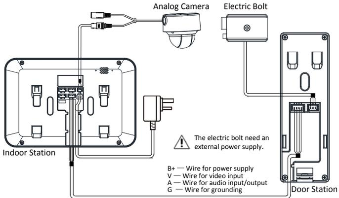
Figure 3-3 Wiring 1 (1 Door Station and 1 Indoor Station)
