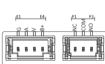
Figure 3-2 Terminals of Door Station
