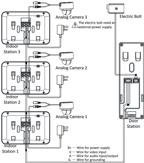
Figure 3-4 Wiring 2 (1 Door Station and 3 Indoor Stations)
