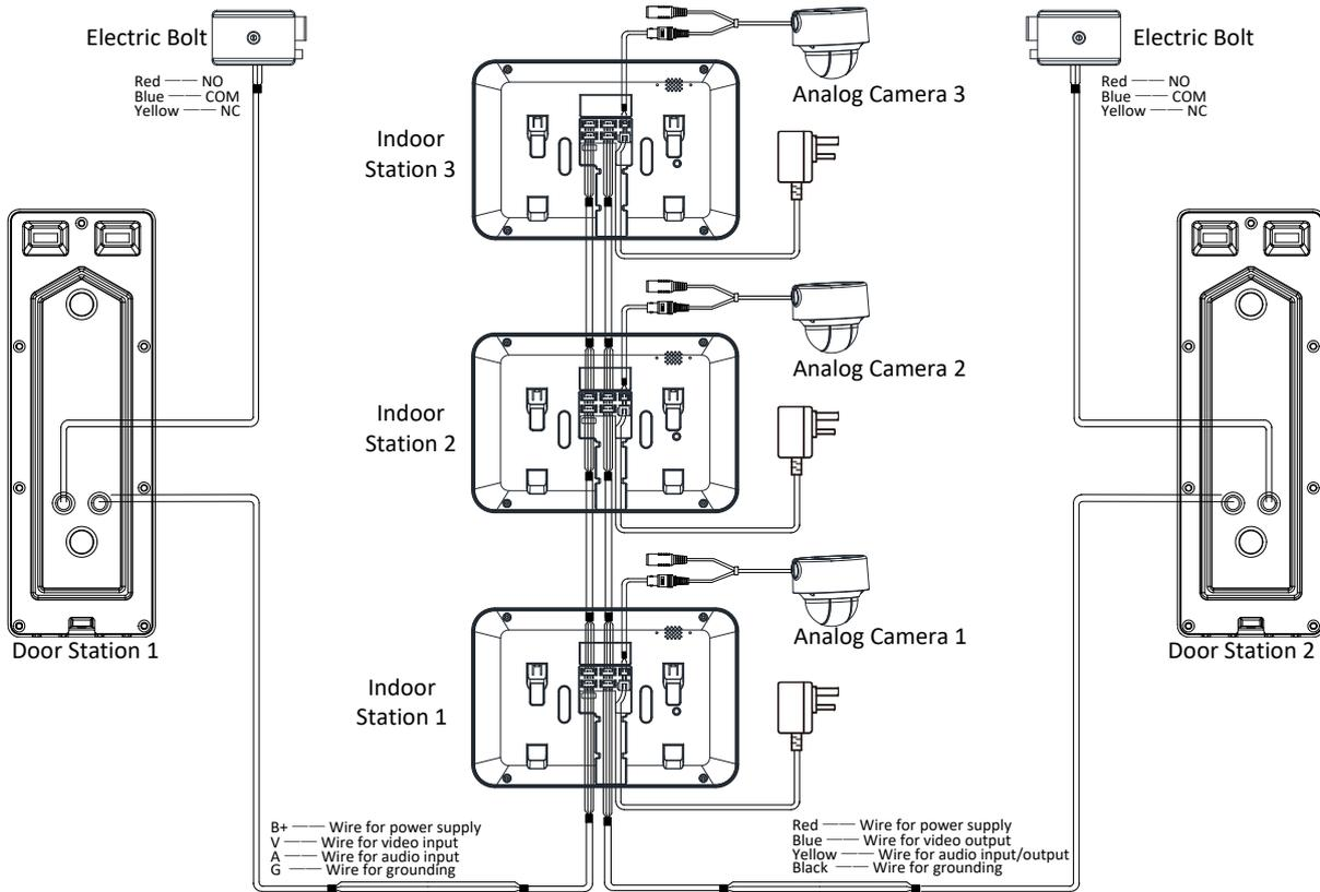
**Figure 3-5 Wiring 3 (2 Door Stations and 3 Indoor Stations)**
