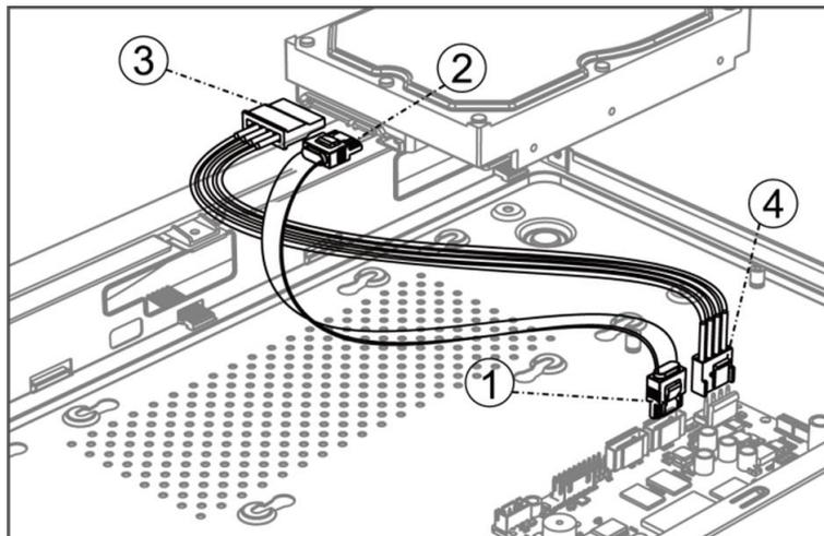
**Figure 1-11 Connect Cables**
