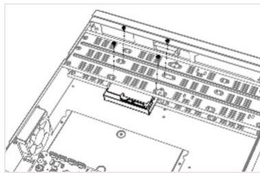
**Figure 1-3 Fix HDD**
