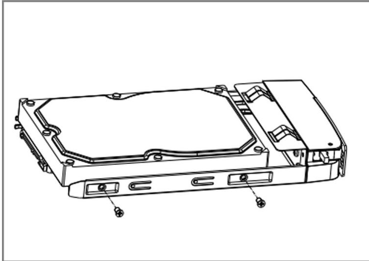
**Figure 1-8 Fix HDD**
