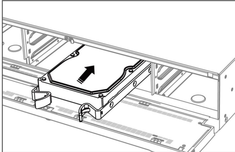
**Figure 1-7 Insert HDD**
