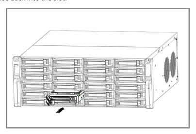
Figure 1-9 Push HDD Case into Slot
