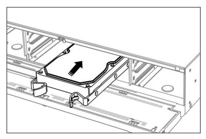
Figure 1-7 Insert HDD
