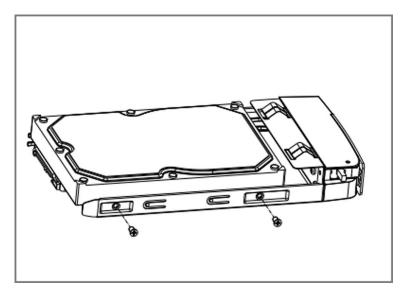
Figure 1-8 Fix HDD
