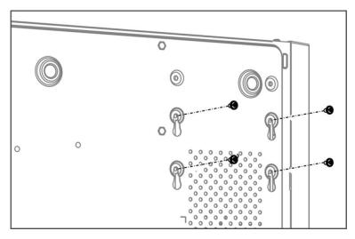
Figure 1-12 Fix HDD to Device Bottom
