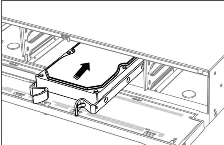
**Figure 1-7 Insert HDD**
