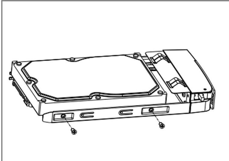
**Figure 1-8 Fix HDD**
