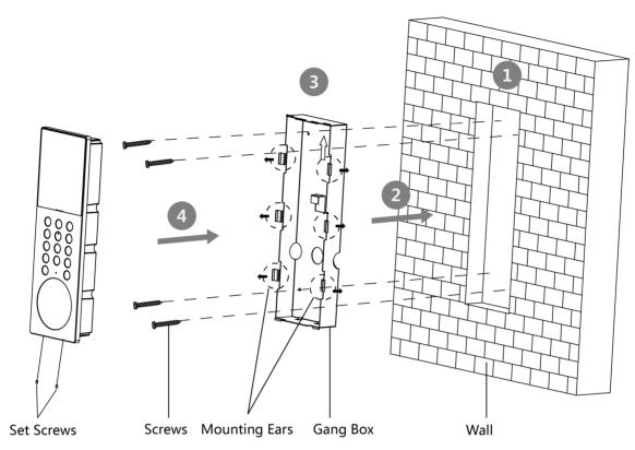
Figure 4-2 Flush Mounting with Gang Box
