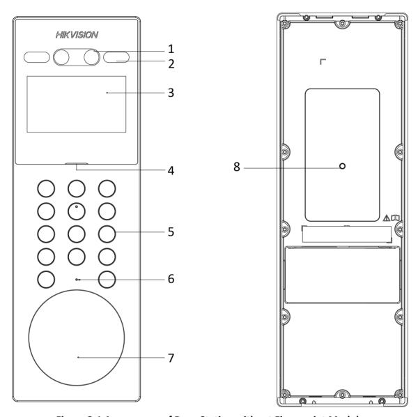
Figure 2-1 Appearance of Door Station without Fingerprint Module
