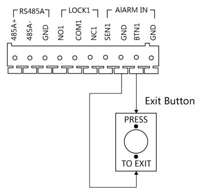
Figure 3-3 Exit Button Wiring
