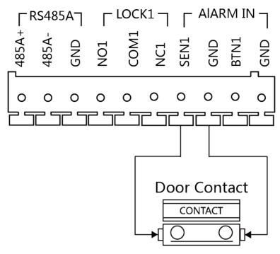
**Figure 3-4 Door Contact Wiring**
