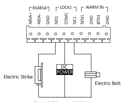
Figure 3-2 Door Lock Wiring
