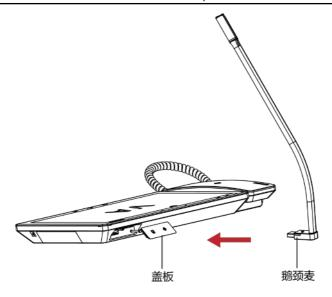
Figure 3-5 Install the Goose Neck Microphone
