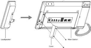
Figure 3-3 Install the Speaker
