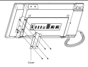
Figure 3-4 Secure the Speaker
