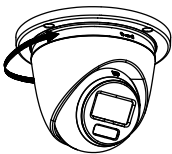
Figure 2-19 Snap Camera into Gang Box
