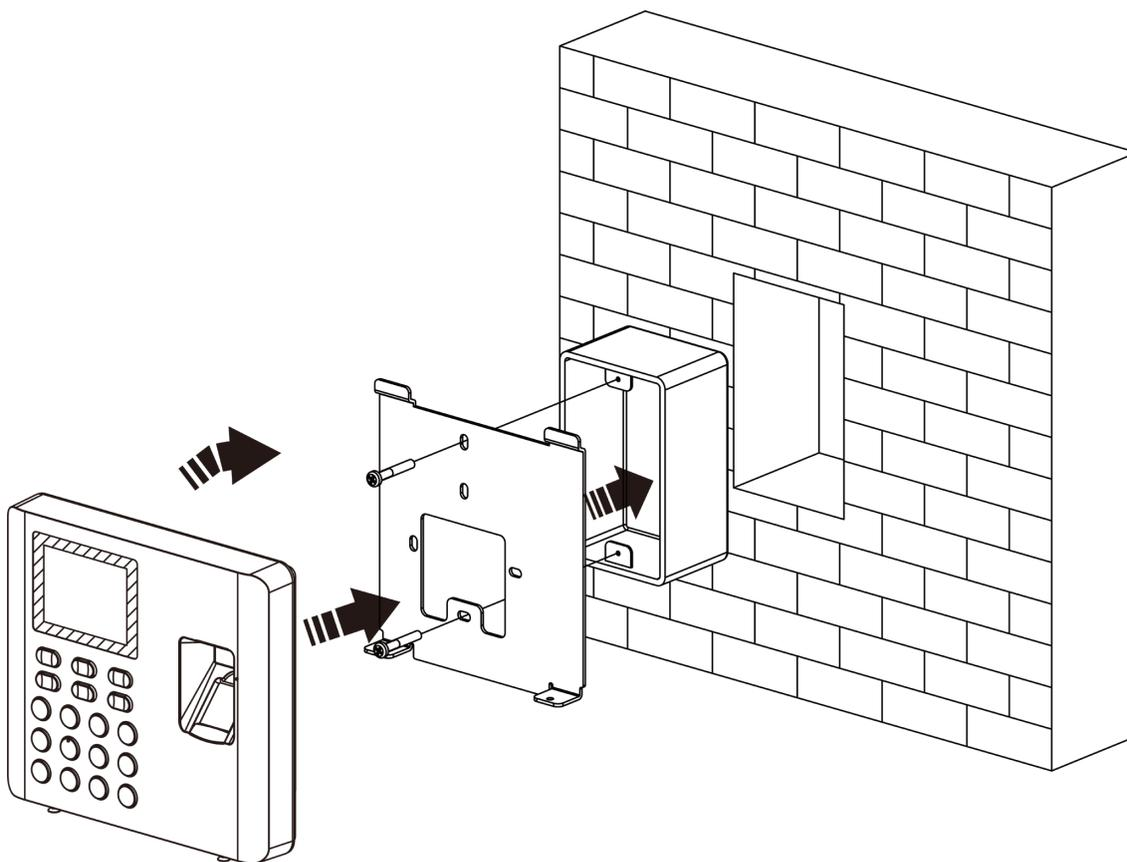
**Figure 3-4 Install Device**
