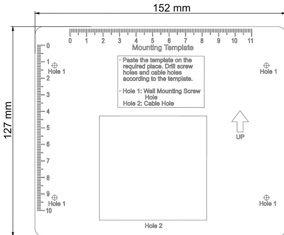
Figure 3-1 Mounting Template
