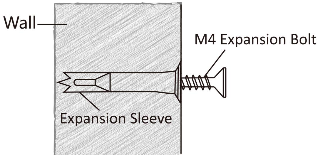
**Figure 3-2 Install Screws**
