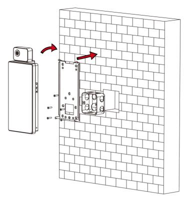
Figure 3-2 Install Device
