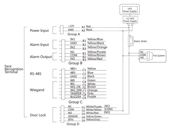
Figure 4-8 Device Wiring
