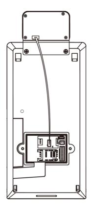
Figure 3-1 Connect Thermographic Module
