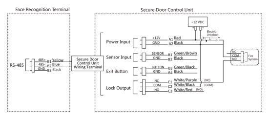
Figure 4-7 Wiring Secure Door Control Unit
