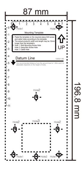
**Figure 3-4 Mounting Template**
