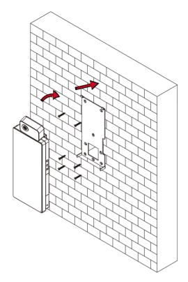
Figure 3-6 Install Device
