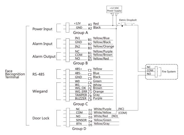
Figure 4-6 Wiring Device
