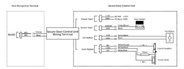
Figure 4-3 Secure Door Control Unit Wiring
