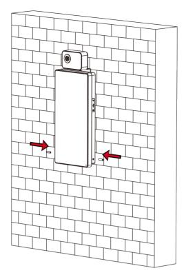
Figure 3-3 Secure Device
