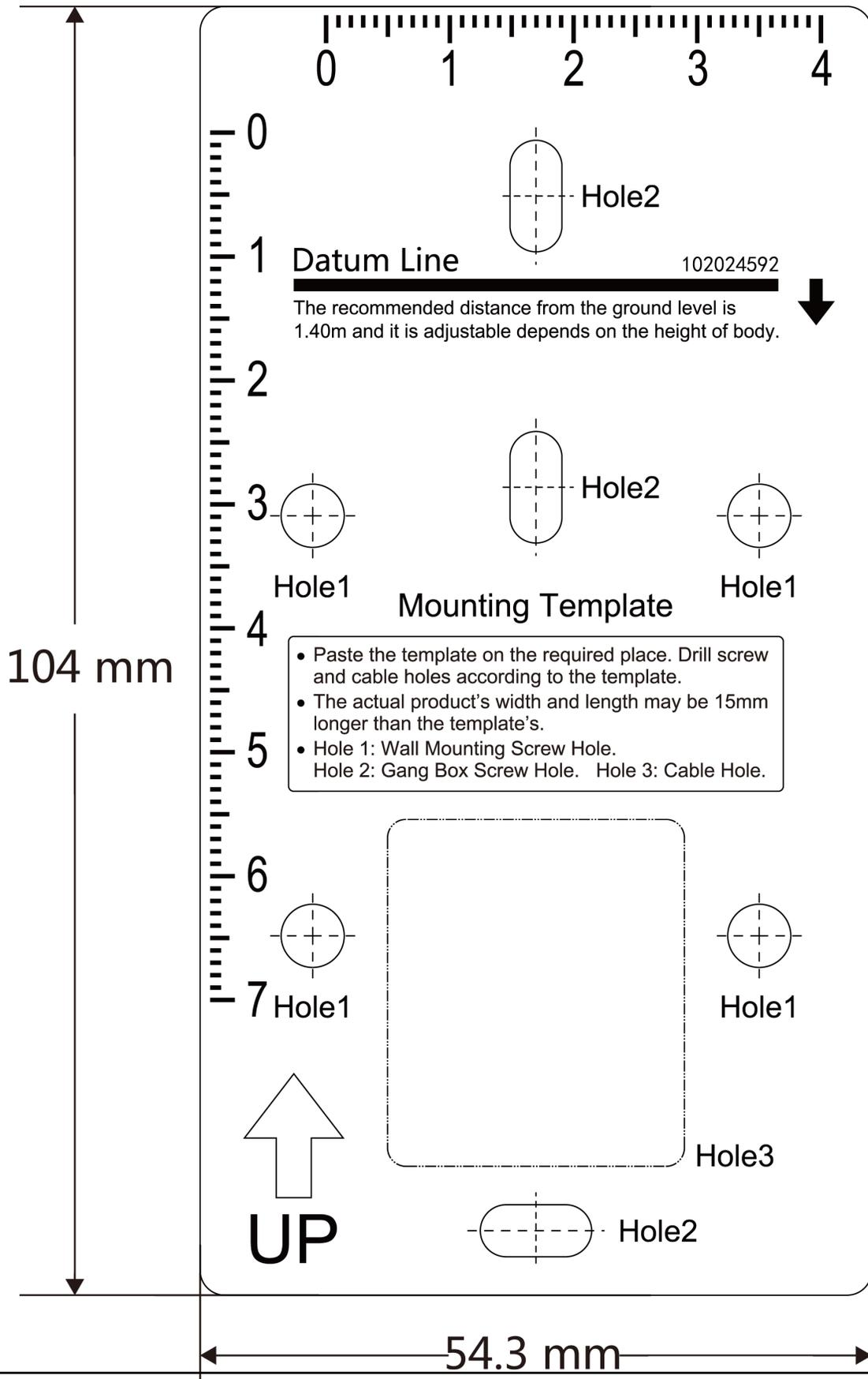
Figure 3-7 Mounting Template
