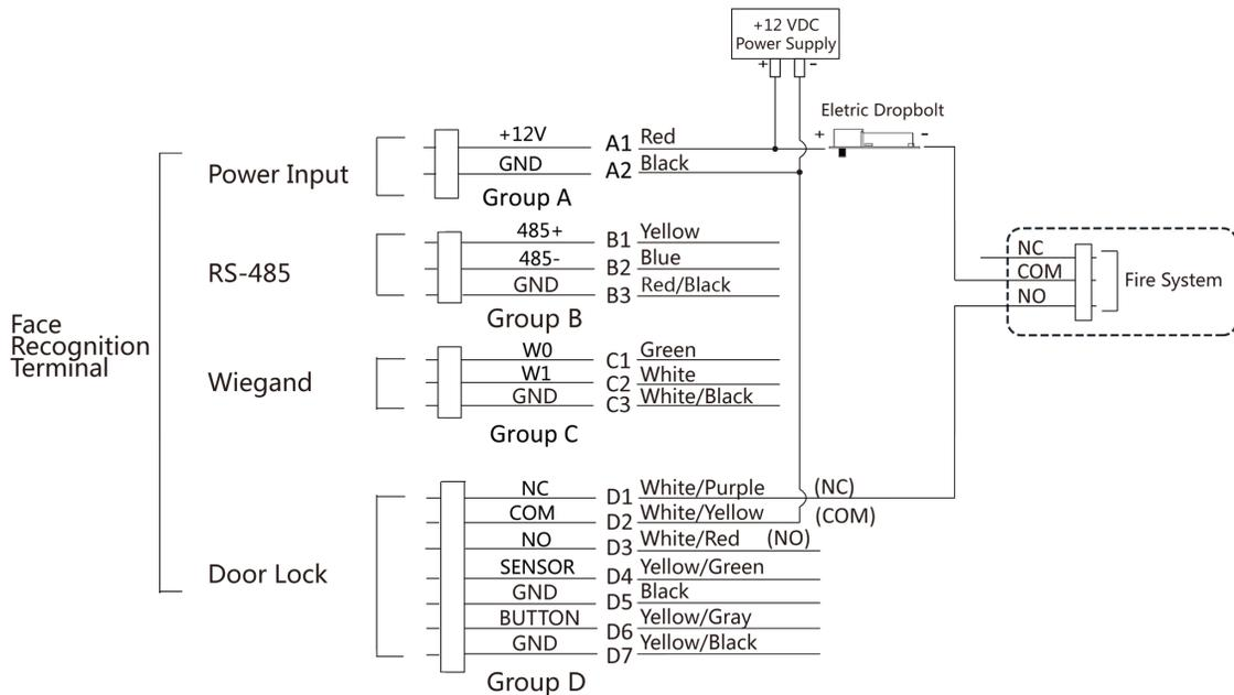
Figure 4-5 Wiring Device
