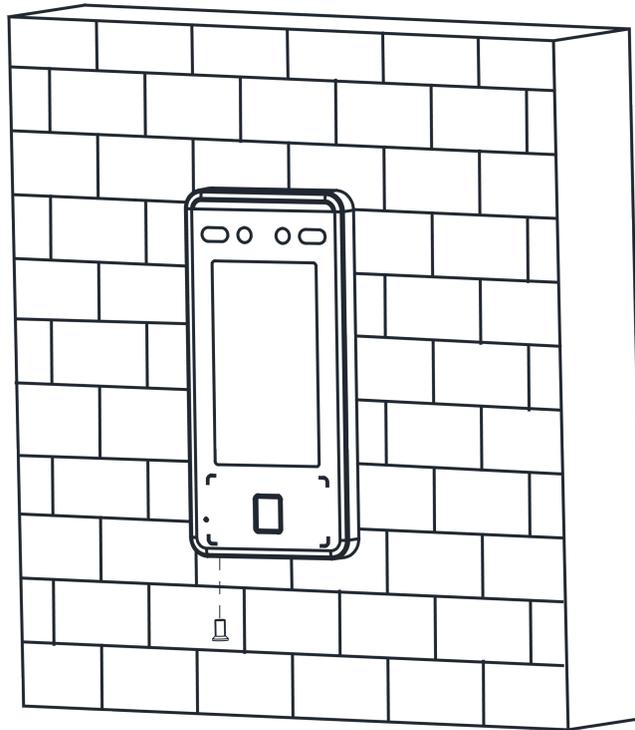
**Figure 3-10 Secure Device**
