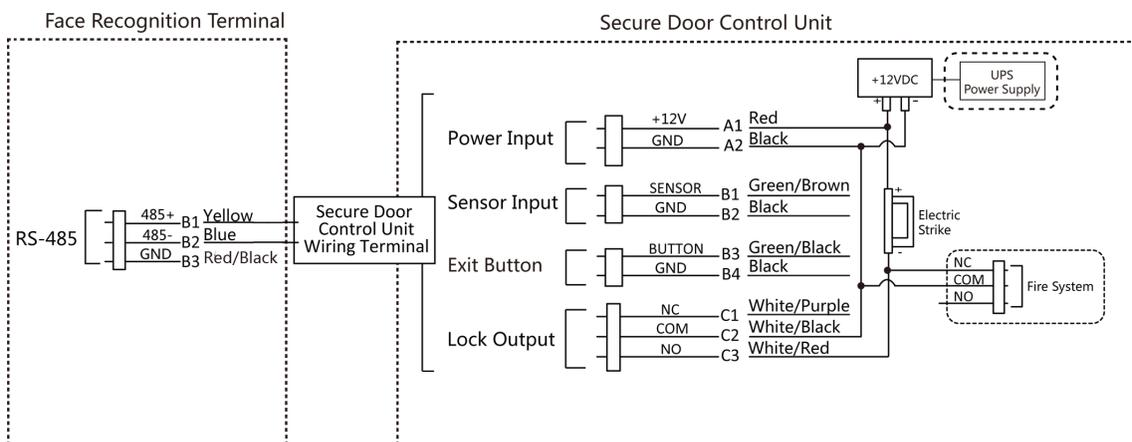
**Figure 4-8 Wiring Diagram**
