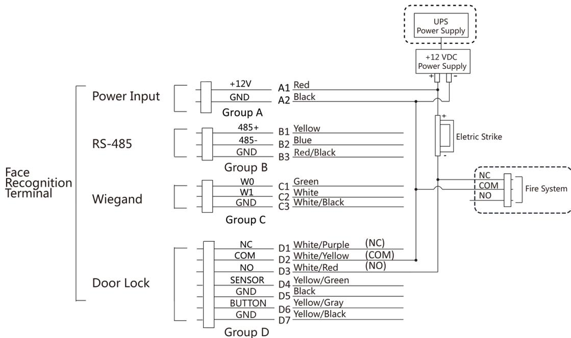
**Figure 4-7 Device Wiring**
