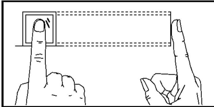
You should press your finger on the scanner horizontally. The center of your scanned finger should align with the scanner center.
