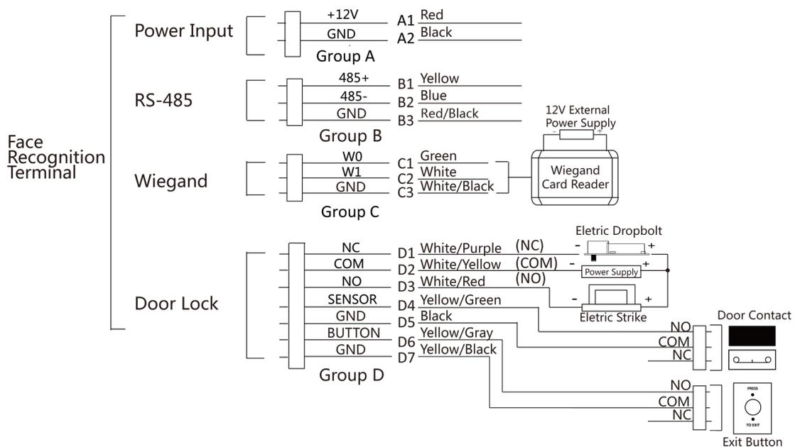
Figure 4-1 Device Wiring
