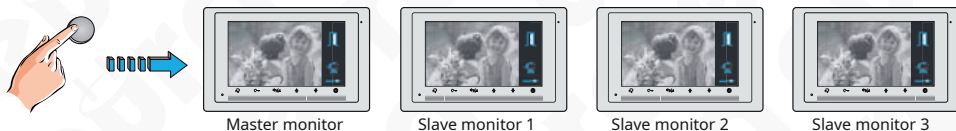
Fig. 16. The function of displaying the preview from the external cassette simultaneously on several monitors
