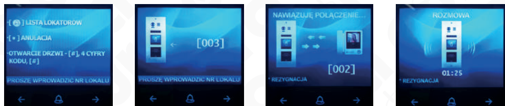
Fig. 26. Calling a locator from the VXA-64A5 keyboard module
