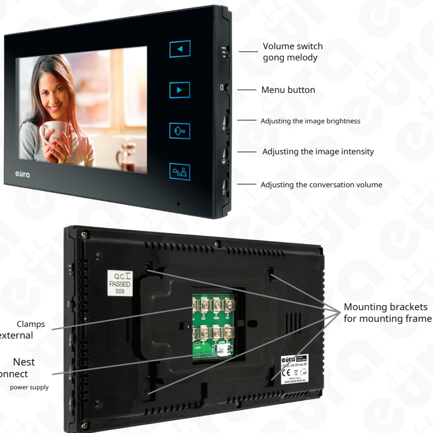
Fig. 1. Construction of the VDA-09A3 monitor
