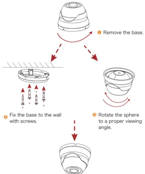
④ Rotate into the base to complete the installation.
