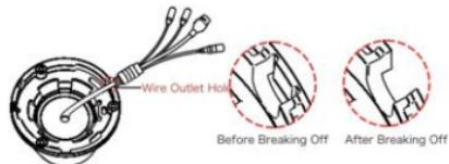
③ Break off the wire outlet hole on the base with dental plier and fix the wire harness to the wire outlet hole.
