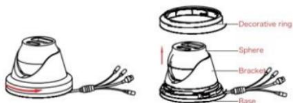
① Rotate and then remove the decorative ring upward.
