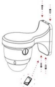
① Loosen 2 screws to separate the bracket from the camera body.
