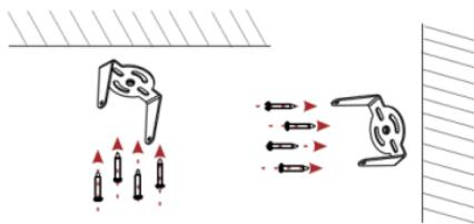
② Use 4 screws to fix the bracket to the ceiling or fix it to the side wall.
