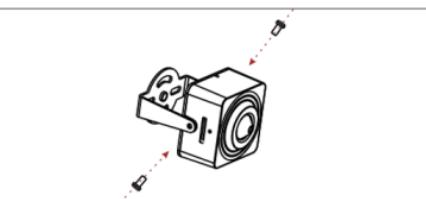
③ Use two screws to fix the camera body and the bracket together. Please do not tighten. Please screw on after adjusting the viewing angle.
