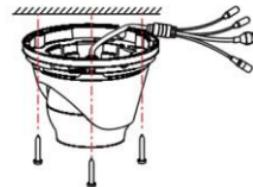
④ Fix the camera to the wall with screws.
