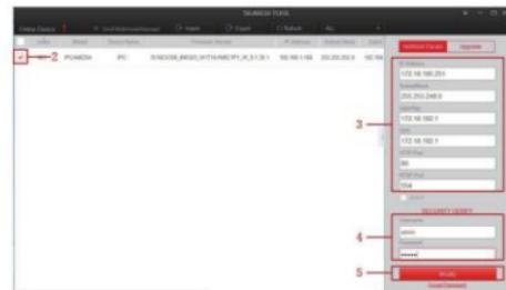
Step 6: Click [Refresh] to search for the modified IP address and the network configuration is successful.
