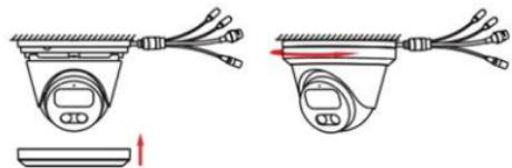
⑥ Put the decorative ring upward and rotate it tightly to complete the installation.
