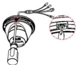
⑤ Rotate the sphere to a proper viewing angle and tighten the screws.
