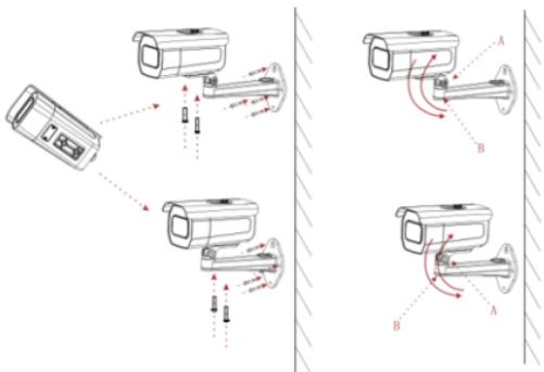
① Fix the camera to the bracket with screws. The bracket head can be pre-mounted or post-mounted, and then fixed to the wall with screws.
