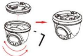
③ Rotate the sphere to the proper viewing angle, snap the groove of the base, and tighten the screws on the side to complete the installation.
