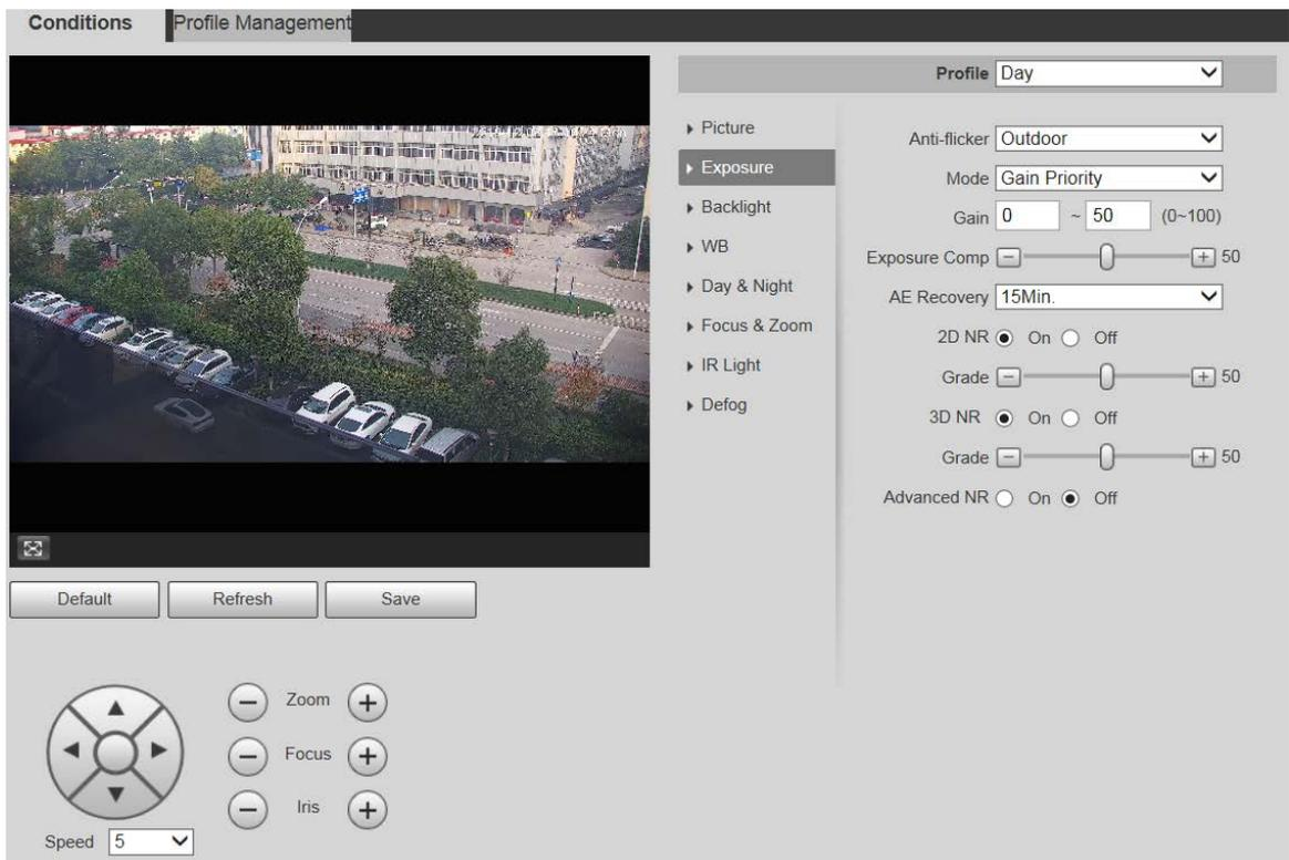
Figure 5-6 Exposure—manual mode
