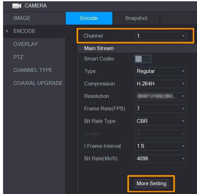
**Step 4** On the **More Setting** interface, enable **Audio Encode** function and then configure the audio settings. In the **Audio Format** list, leave it as default; in the **Audio Source** list, select **HDCVI**.
