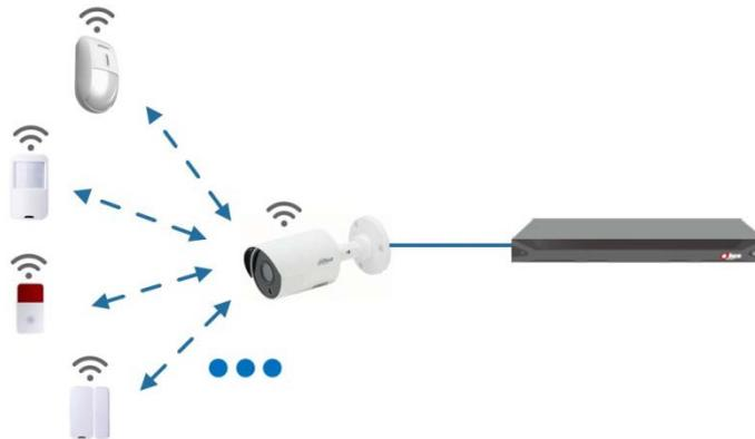
Connect the wireless node devices to XVR with gateway camera and then configure parameters.
