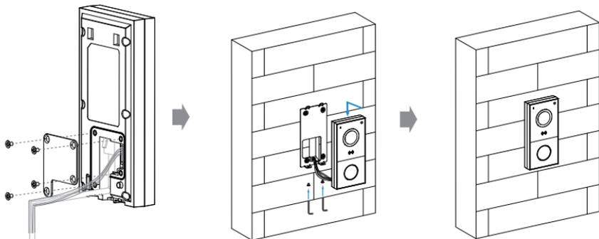
Connect the wires to the interface of the device as needed (for details, refer to "Device Wiring"). After arranging the wires, tighten the back cover using four M3x4 screws to the device.
