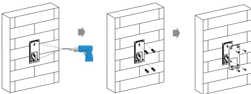
According to the position of the reserved wires on the wall, stick the wall-mounting template vertically to ensure that the wires can come out of the shadow position of template. Drill (6 mm drill bit required) four screw holes with a depth of 25mm in the screw holes of the template.
